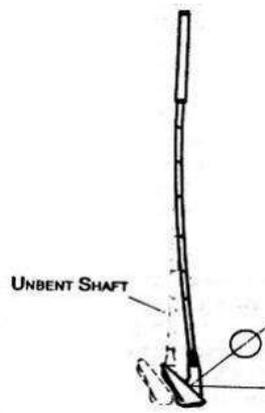
(a) Bending in plane of swing (lead/lag)
