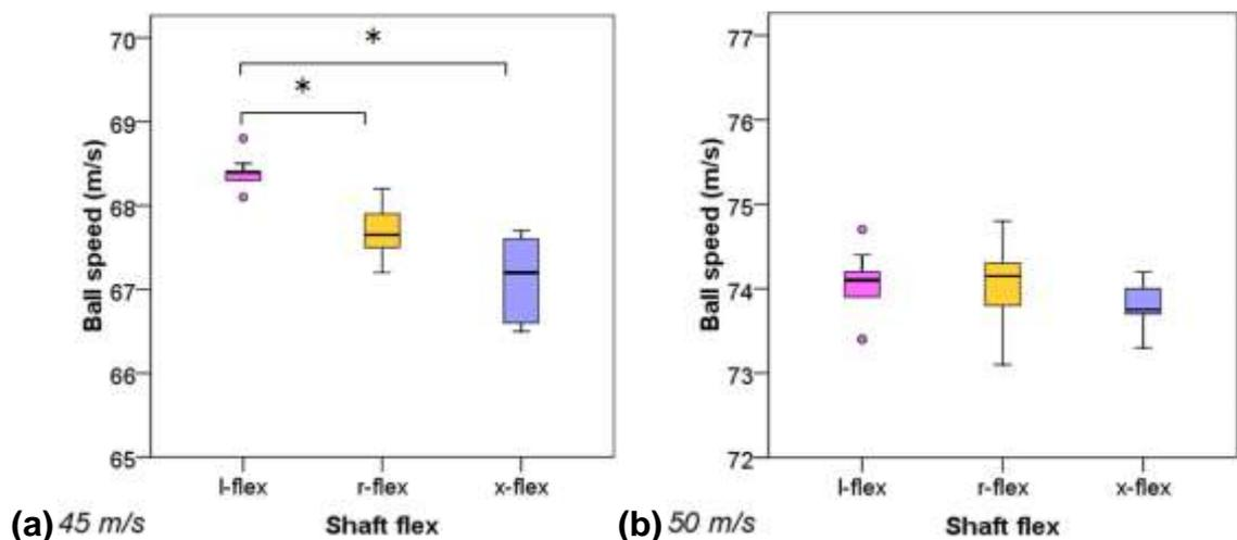
**Figure 62: Ball speeds measured for club head speeds of 45 m/s (a) and 50 m/s (b). Shaft pairs with significant differences are marked with “\*”. Dots indicate outliers (only present in the l-flex data sets).**
