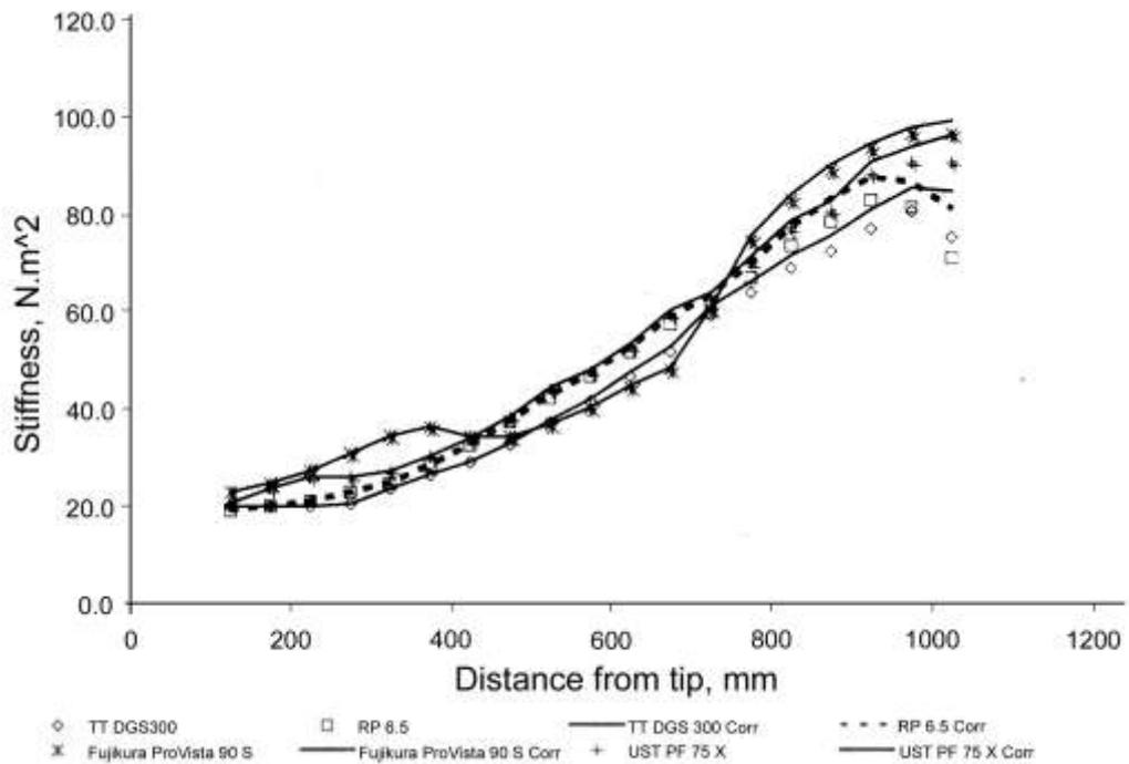
**Figure 8: Stiffness profiles for four different golf shafts before and after applying a correction for measurement errors. It can be seen that each shaft has characteristic stiffness variations between tip and butt end (adapted from Mase, 2004, p. 520).**
