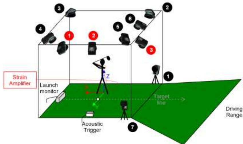
**Figure 38: Test set-up. Numbers in black circles denote positions of the body motion capture system, numbers in red circles denote cameras pertaining to the impact location motion capture system.**
