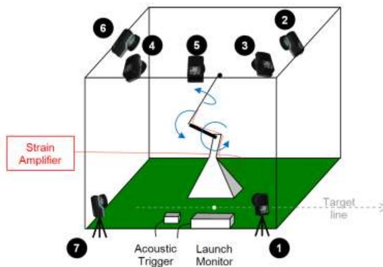
**Figure 53: Setup for robot testing. ①-⑦ denote motion capture cameras.**
