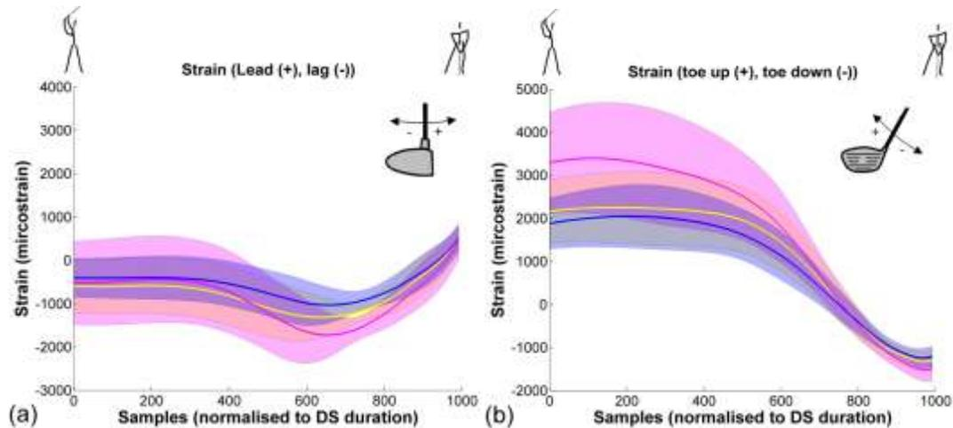
**Figure 36: Mean strain patterns in lead/lag direction (a) and toe up/down direction (b). Lines represent mean strain for all subjects for the I-flex (pink), r-flex (yellow) and x-stiff (blue) shaft. Shaded areas indicate  $\pm 1$  SD.**
