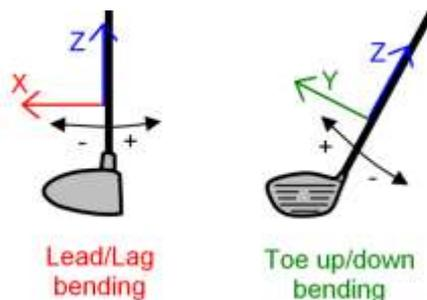
**Figure 23: Reference system and nomenclature for strain measurements.**
