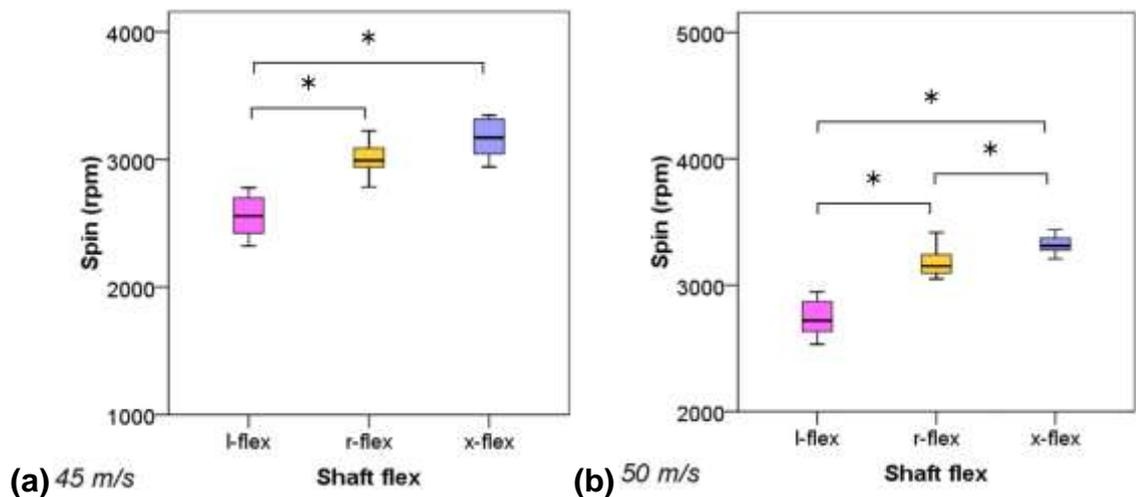
**Figure 64: Spin rates measured for club head speeds of 45 m/s (a) and 50 m/s (b). Shaft pairs with significant differences are marked with “\*”.**
