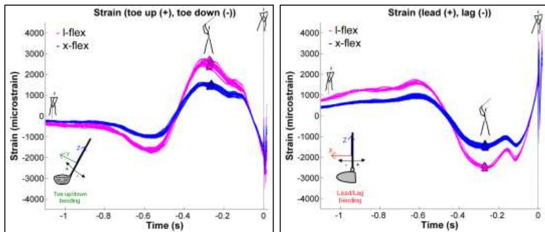
**Figure 48: Typical strain patterns (all swings shown were performed by one player). The transition from backswing to downswing is marked with a  $\Delta$  symbol.**
