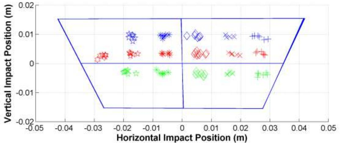
**Figure 30: Face mapping results. The rows of grid points (blue, red, green) were separated by 6 mm, columns by 11 mm.**
