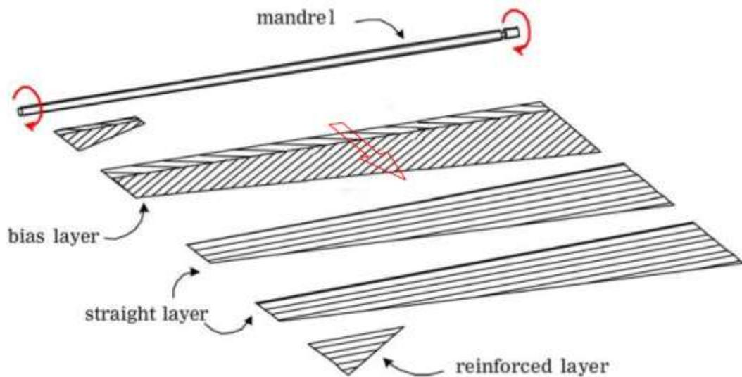
**Figure 3: Lay-up process for sheet-laminated shafts (adapted from Cheong, Kang, & Jeong, 2006, p. 465).**
