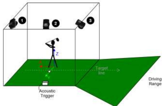
**Figure 27: Setup of custom club head tracking system (cameras: ①-③).**
