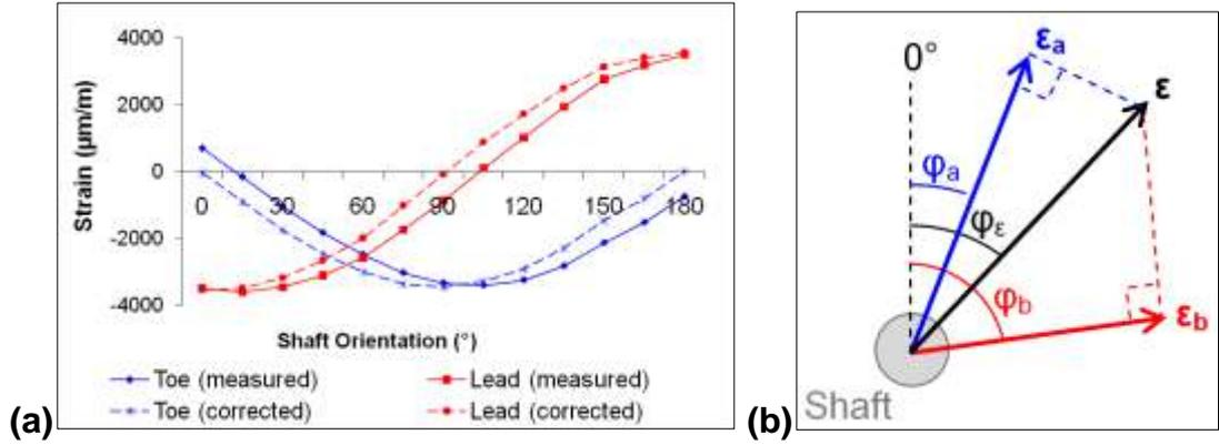
**Figure 25: (a) Example results from strain gauge calibration. (b) Shaft cross section with nomenclature for calibration procedure.**
