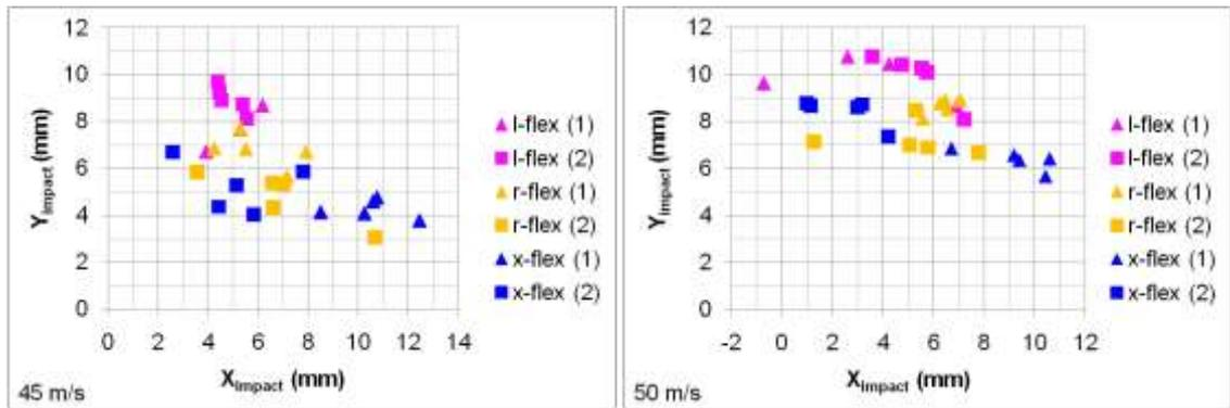
**Figure 61: Impact positions for different shaft conditions for impact speeds of approximately 45 m/s (left) and 50 m/s (right). Club numbers (1) and (2) refer to the first and second club replicate, respectively.**
