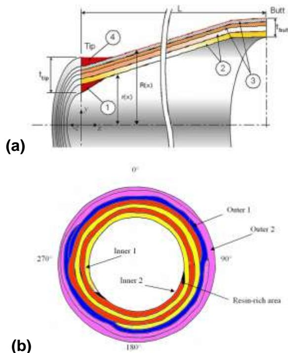
**Figure 4: (a) Typical composition of a sheet-laminated shaft from a number of layers<sup>2</sup> of carbon/epoxy pre-pregs (adapted from Cheong, Kang, & Jeong, 2006, p. 469). (b) Resulting lay-up of carbon/epoxy layers. Fibres of the inner layer are typically oriented at  $\pm 45^\circ$ , fibres of the outer layer at  $0^\circ$  (adapted from Huntley, 2007, p. 140).**
