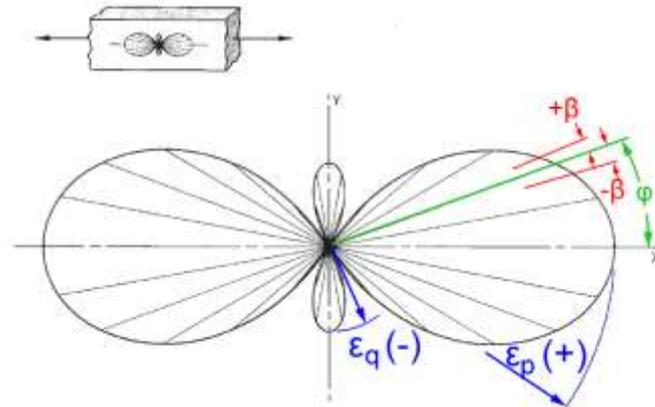
**Figure 24: Strain field created by a uniaxial stress field.  $\varepsilon_p$  and  $\varepsilon_q$  denote the maximum and minimum principal strains,  $\varphi$  is the intended alignment angle of the strain gauge and  $\beta$  is the alignment error (mod. from Vishay, 2007).**
