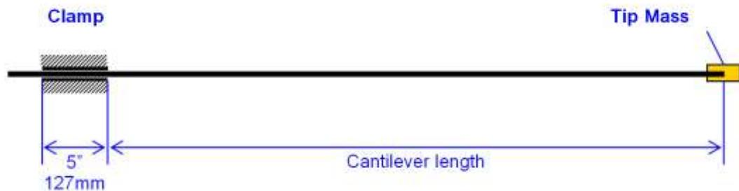
**Figure 19: Set-up of frequency test.**
