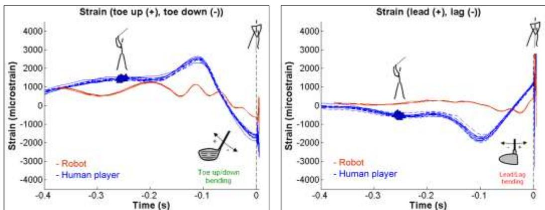
**Figure 57: Comparison of human and robotic shaft loading for two clubs with identical stiffness ratings (x-flex). Stick figures indicate the time of the transition from backswing to downswing and impact for the human player.**
