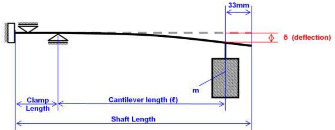
**Figure 20: Set-up of rigidity test.**
