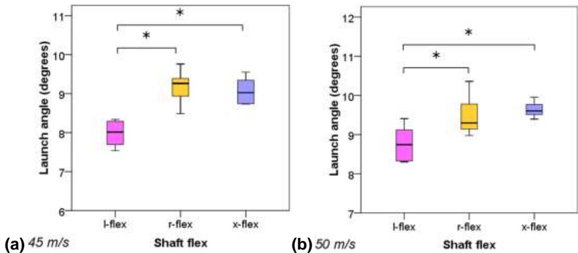
**Figure 63: Launch angles measured for club head speeds of 45 m/s (a) and 50 m/s (b). Shaft pairs with significant differences are marked with “\*”.**
