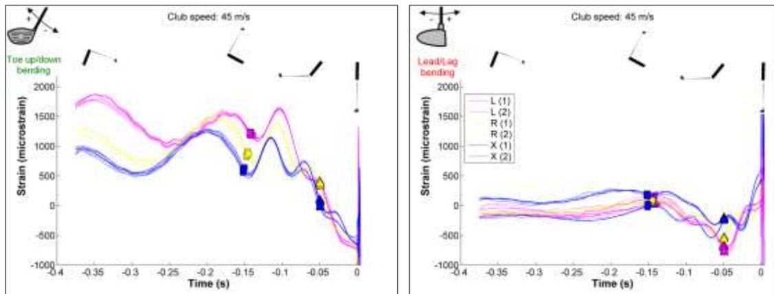
**Figure 58: Strain patterns recorded for robot swings performed with an impact speed of approximately 45 m/s. Symbols indicate wrist release (□) and grip-horizontal event (△). Club numbers (1) and (2) refer to the first and second club replicate, respectively,**
