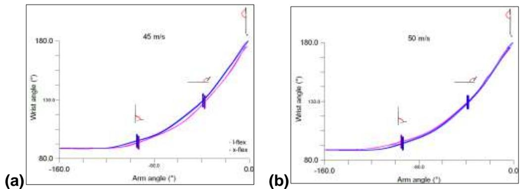
**Figure 60: Wrist angle as a function of arm angle for swings with a club head speed of 45 m/s (a) and 50 m/s (b). Plot shows a mean curve for all recorded swings. Standard deviations are shown as shaded areas but are barely visible due to the consistency of the robot. Vertical lines indicate swing events as defined in Section 7.1.4.**
