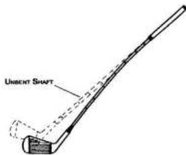
(c) Bending perpendicular to plane of swing (toe-up/down)
