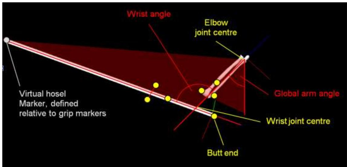
**Figure 40: Definition of four-point wrist angle and position of virtual offset marker placed at tip end of shaft.**
