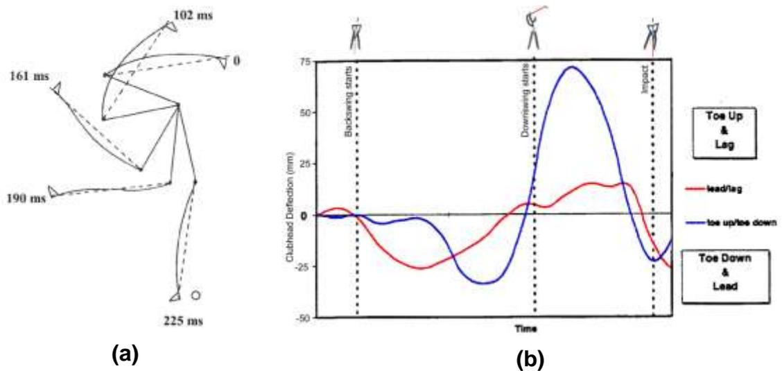
**Figure 1: Shaft behaviour during a typical golf swing: (a) simulation of shaft bending according to Milne & Davis' (1992) measurements (bending exaggerated by a factor of 5) (adapted from Penner, 2003, p. 158); (b) bending of the shaft during a typical golf swing (adapted from Newman, Clay, & Strickland, 1997, p. 369).**
