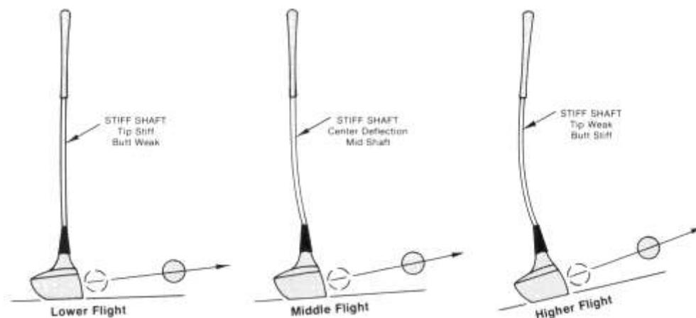
**Figure 14: Expected effect of shaft stiffness distribution on launch angle (adapted from Maltby, 1995, p. 416).**
