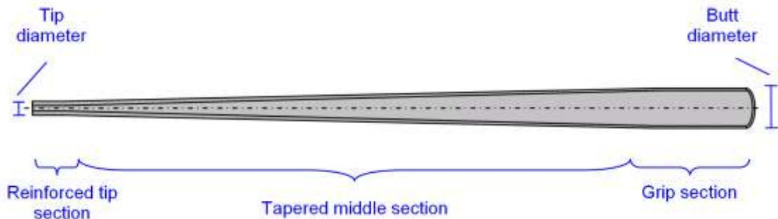
**Figure 6: Typical shaft geometry (cross section). Shaft diameter is exaggerated relative to length for clarity (based on data presented in Huntley, 2007).**
