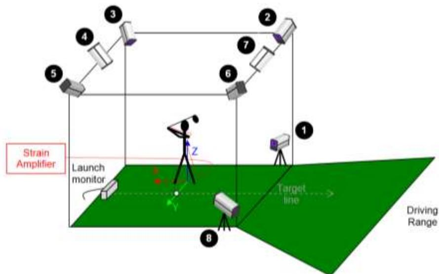
**Figure 31: Set-up for player testing (cameras: ①-⑧).**
