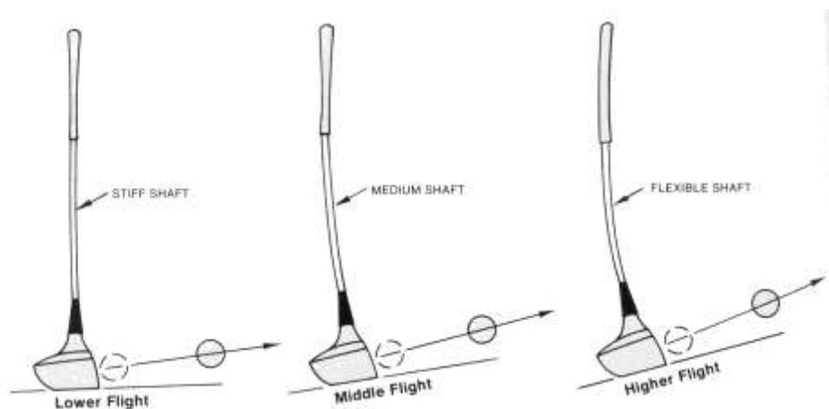
**Figure 15: Expected effect of shaft stiffness on launch angle (adapted from Maltby, 1995, p. 414).**
