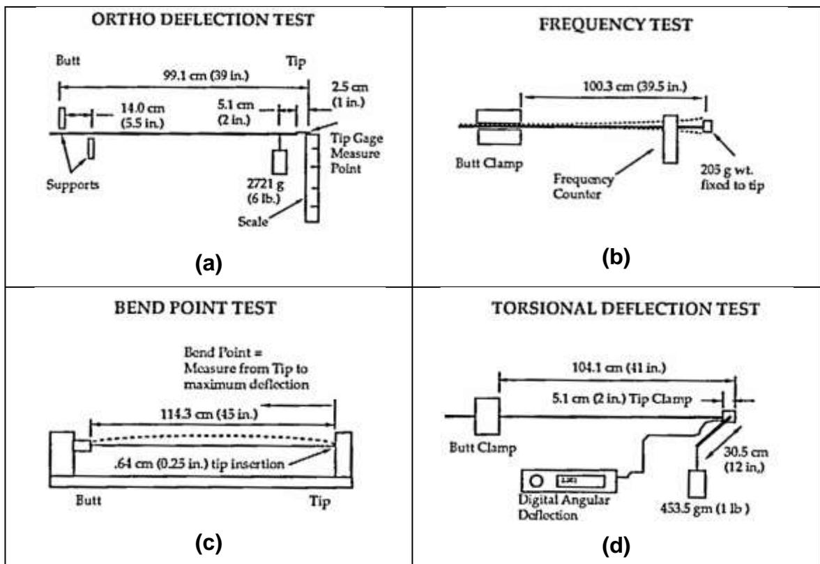
Figure 9: Four static shaft tests (adapted from Howell, 1992, p. 1395).
