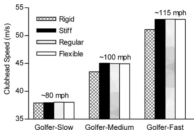
**Fig. 6** Clubhead speed at impact for the 12 optimized golfer-club models. The Rigid club condition represents a shaft with infinite stiffness and, as such, does not bend during the downswing
