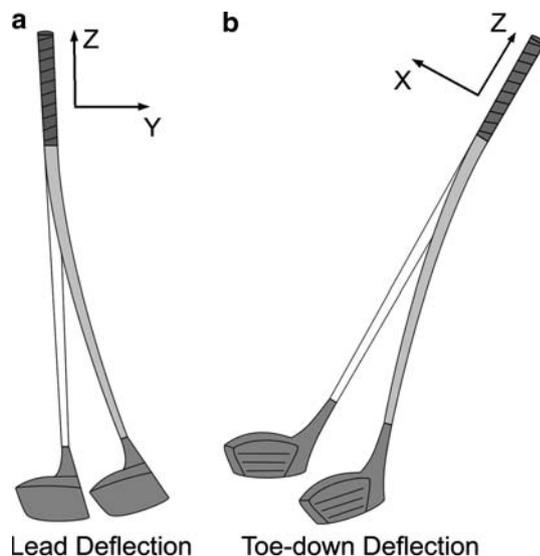
**Fig. 1** The modeled shafts were capable of deflecting about two axes. **a** Deflection along the *Y* axis represents lead/lag motion. **b** Deflection along the *X* axis represents toe-up/toe-down motion
