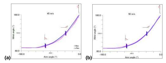
Figure 60: Wrist angle as a function of arm angle for swings with a club head speed of 45 m/s (a) and 50 m/s (b). Plot shows a mean curve for all recorded swings. Standard deviations are shown as shaded areas but are barely visible due to the consistency of the robot. Vertical lines indicate swing events as defined in Section 7.1.4.
