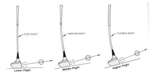
Figure 15: Expected effect of shaft stiffness on launch angle (adapted from Maltby, 1995, p. 414).
