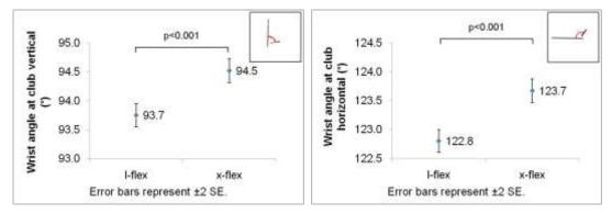
Figure 50: Estimated marginal means for planar wrist angle at the grip-vertical and the grip-horizontal events.
