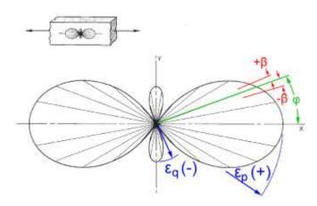
Figure 24: Strain field created by a uniaxial stress field.  $\varepsilon_{\rho}$  and  $\varepsilon_{q}$  denote the maximum and minimum principal strains,  $\varphi$  is the intended alignment angle of the strain gauge and  $\beta$  is the alignment error (mod. from Vishay, 2007).
