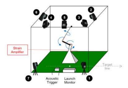
Figure 53: Setup for robot testing. **0-** denote motion capture cameras.
