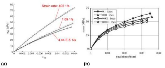
Figure 5: Stress(σ)-strain(ε) graphs for composites loaded at different strain rates: (a) based on micromechanical modelling (Zhu,
