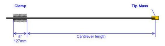
Figure 19: Set-up of frequency test.
