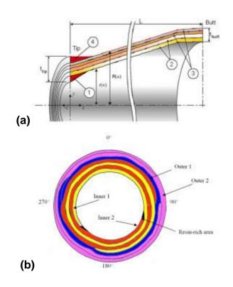
Figure 4: (a) Typical composition of a sheet-laminated shaft from a number of layers<sup>2</sup> of carbon/epoxy pre-pregs (adapted from Cheong, Kang, & Jeong, 2006, p. 469). (b) Resulting lay-up of carbon/epoxy layers. Fibres of the inner layer are typically oriented at ±45°, fibres of the outer layer at 0° (adapted from Huntley, 2007, p. 140).
