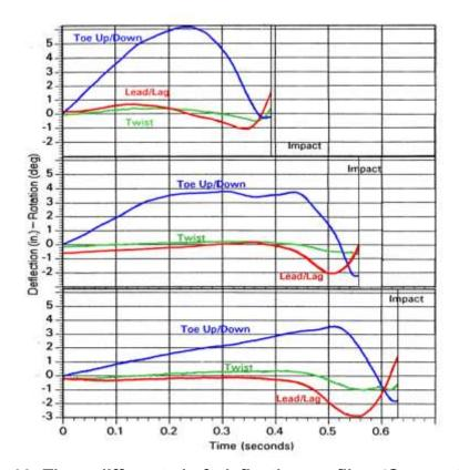
Figure 16: Three different shaft deflection profiles. 'One-peak' (top), 'double-peak' (middle) and 'ramp-like' (bottom) (mod. from Butler & Winfield, 1994, pp. 261-262). Positive values correspond to toe-up, lead and face-close deflection, negative values to toe-down, lag and face-open deflection<sup>7</sup>.
