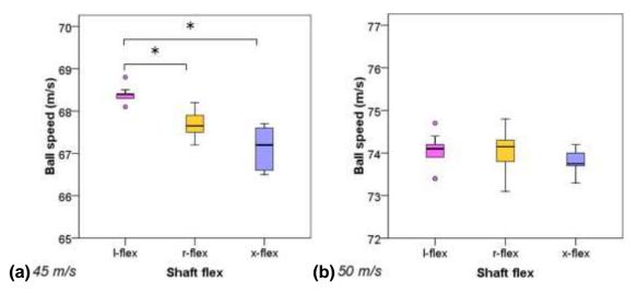
Figure 62: Ball speeds measured for club head speeds of 45 m/s (a) and 50 m/s (b). Shaft pairs with significant differences are marked with '\*'. Dots indicate outliers (only present in the I-flex data sets).
