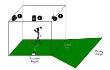
Figure 27: Setup of custom club head tracking system (cameras: **0**-**6**).
