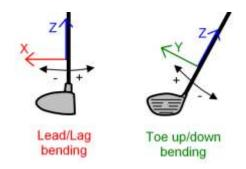
Figure 23: Reference system and nomenclature for strain measurements.
