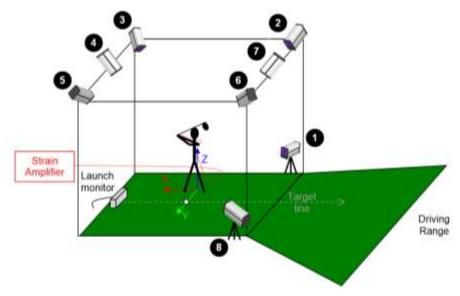
Figure 31: Set-up for player testing (cameras: **0**-**8**).
