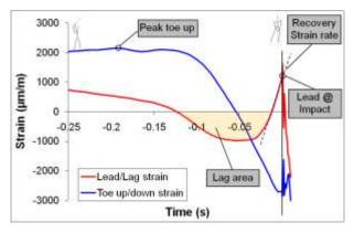
Figure 26: Definition of characteristic downswing strain parameters.
