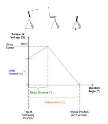
Figure 54: Control settings of the robot (based on Golflabs, 2007).
