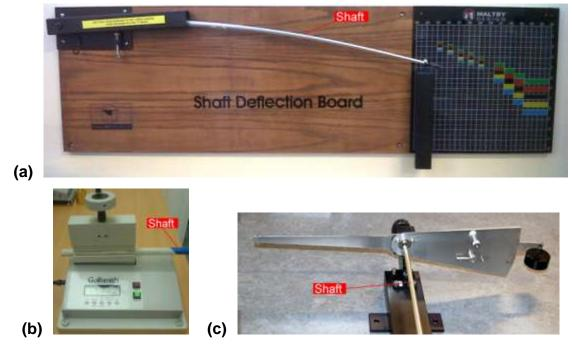
Figure 10: Commercial shaft test equipment. (a) Deflection board (Maltby Design, USA), (b) Frequency analyser (Golfsmith, USA), (c) Torsion test (Golfmechanix, Taiwan ROC).
