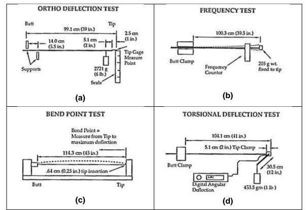
Figure 9: Four static shaft tests (adapted from Howell, 1992, p. 1395).
