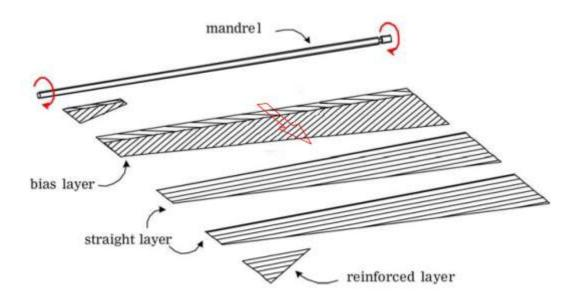
Figure 3: Lay-up process for sheet-laminated shafts (adapted from Cheong, Kang, & Jeong, 2006, p. 465).
