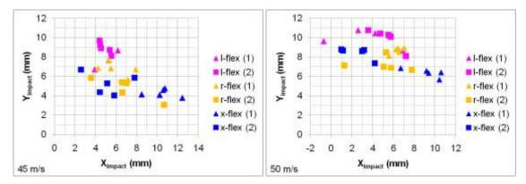
Figure 61: Impact positions for different shaft conditions for impact speeds of approximately 45 m/s (left) and 50 m/s (right). Club numbers (1) and (2) refer to the first and second club replicate, respectively.
