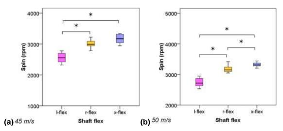
Figure 64: Spin rates measured for club head speeds of 45 m/s (a) and 50 m/s (b). Shaft pairs with significant differences are marked with '\*'.
