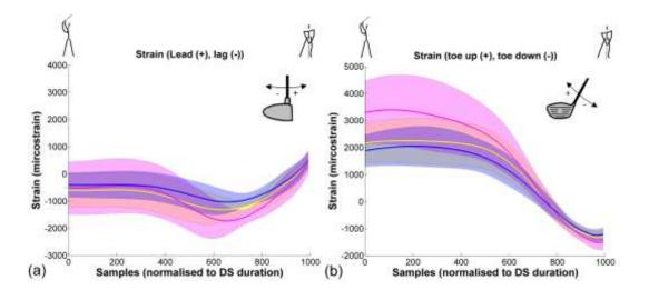
Figure 36: Mean strain patterns in lead/lag direction (a) and toe up/down direction (b). Lines represent mean strain for all subjects for the l-flex (pink), r-flex (yellow) and x-stiff (blue) shaft. Shaded areas indicate ±1 SD.
