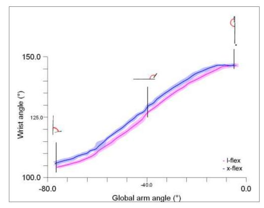
Figure 51: Example for wrist angle joint history for one subject. For clarity, wrist angle is plotted as a function of global arm angle rather than time (see Figure 40 for angle definitions). Shaded areas indicate  $\pm 1$  SD.
