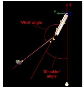
Figure 55: Definition of shoulder and wrist angle for the golf robot. The zaxis of the global coordinate system runs perpendicular to the arm.
