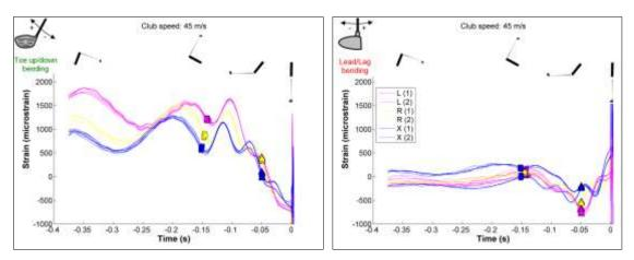
Figure 58: Strain patterns recorded for robot swings performed with an impact speed of approximately 45 m/s. Symbols indicate wrist release ( $\Box$ ) and grip-horizontal event ( $\triangle$ ).Club numbers (1) and (2) refer to the first and second club replicate, respectively,
