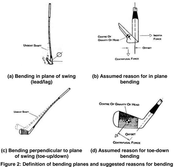
Figure 2: Definition of bending planes and suggested reasons for bending (adapted from Horwood, 1994, p. 249 and 251).
