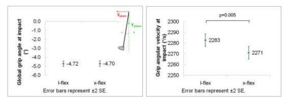
Figure 52: Estimated marginal means for the planar club angle and angular velocity. This angle was calculated after projecting the longitudinal axis of the grip on the x-z-plane (vertical) and is relative to the z-axis.
