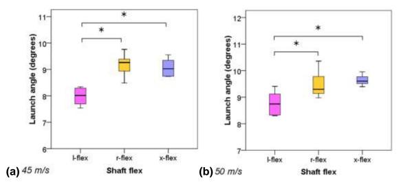
Figure 63: Launch angles measured for club head speeds of 45 m/s (a) and 50 m/s (b). Shaft pairs with significant differences are marked with '\*'.
