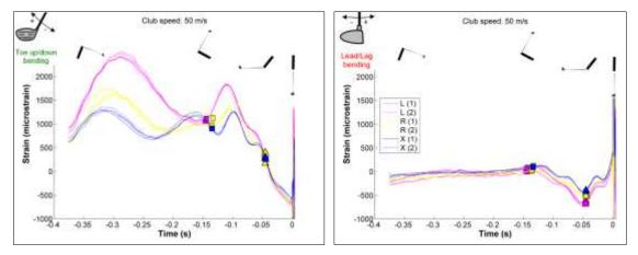
Figure 59: Strain patterns recorded for robot swings performed with an impact speed of approximately 50 m/s. See previous figure for details.
