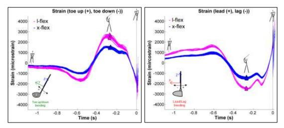
Figure 48: Typical strain patterns (all swings shown were performed by one player). The transition from backswing to downswing is marked with a  $\triangle$  symbol.
