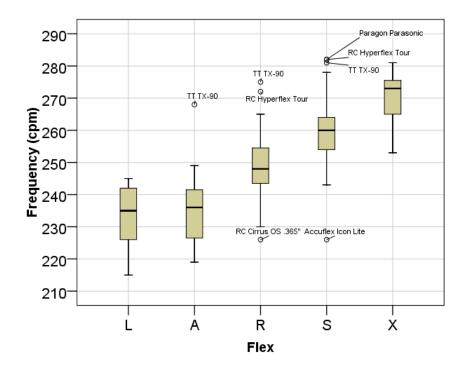
Figure 18: Boxplot showing driver shaft frequency ranges for different flex codes (based on data for 300 driver shafts presented by Summitt, 2000)
