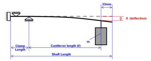
Figure 20: Set-up of rigidity test.
